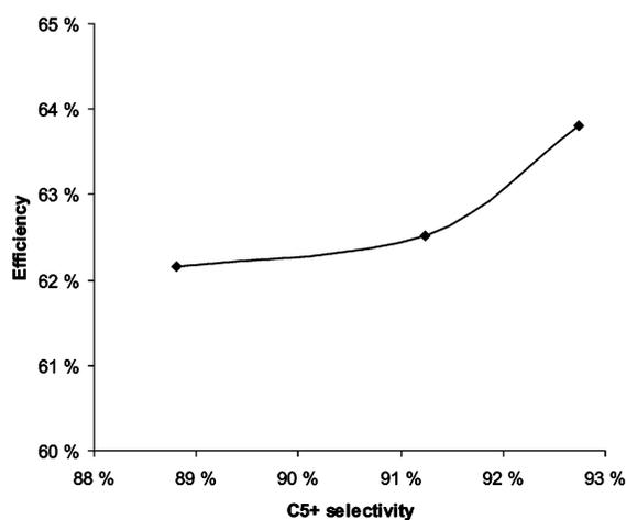
Figure 9. Effect of F-T selectivity on the process efficiency.
