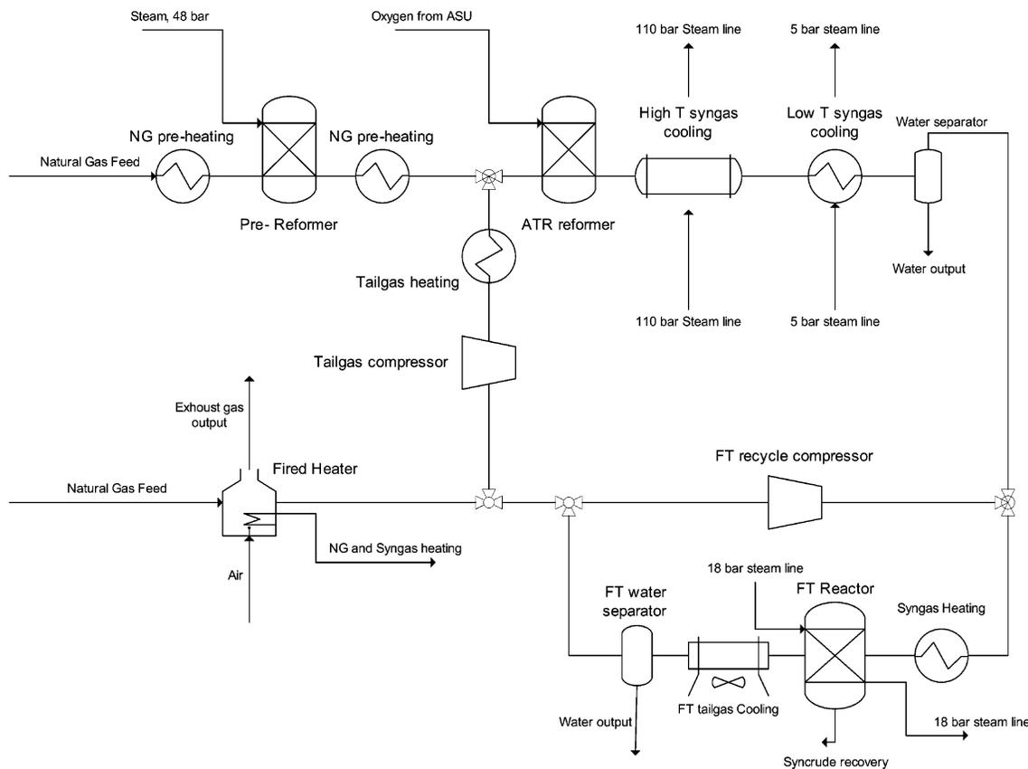
Figure 1. Schematic flowsheet (power plant and ASU not shown).
