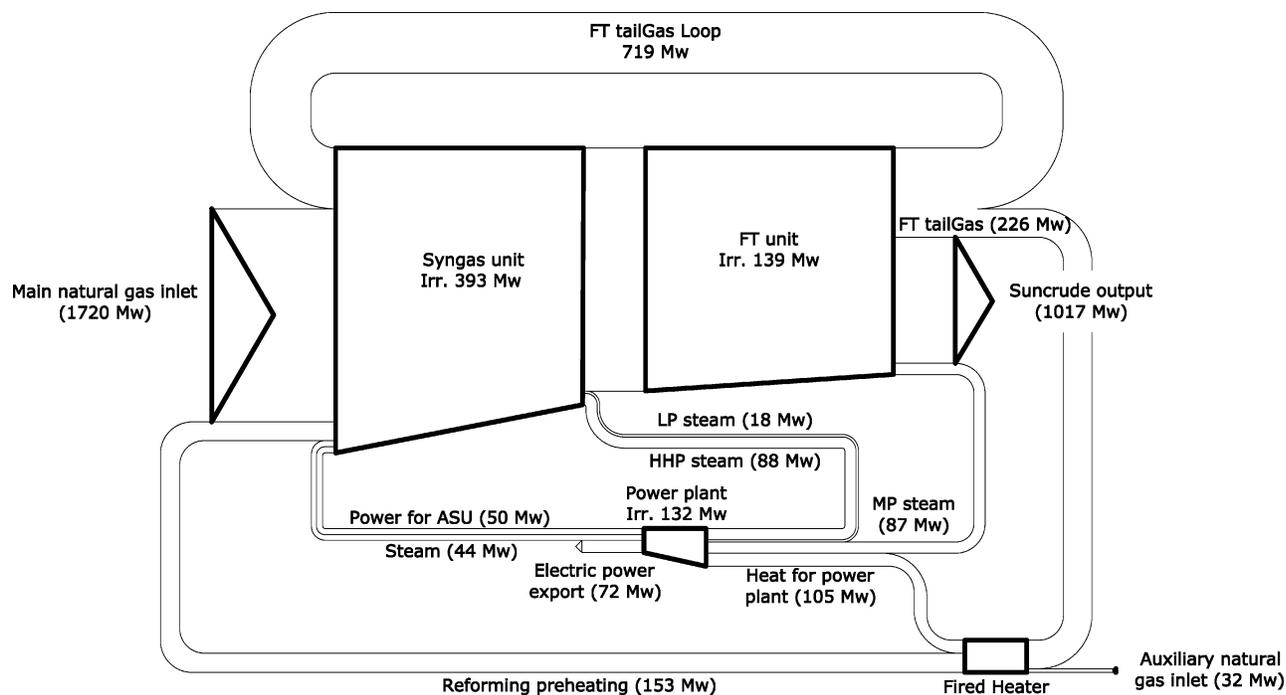
**Figure 6.** Grassman diagram of the GTL process. Streams with exergy below 15 MW are not shown. Fired heater losses are allocated to the power plant and the syngas unit.
