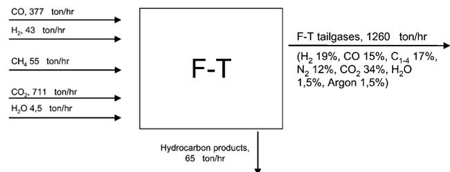
**Figure 4. F–T reactor mass balance.**
