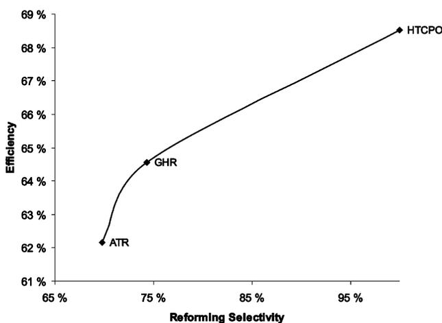
Figure 10. Process efficiency as a function of reforming selectivity.
